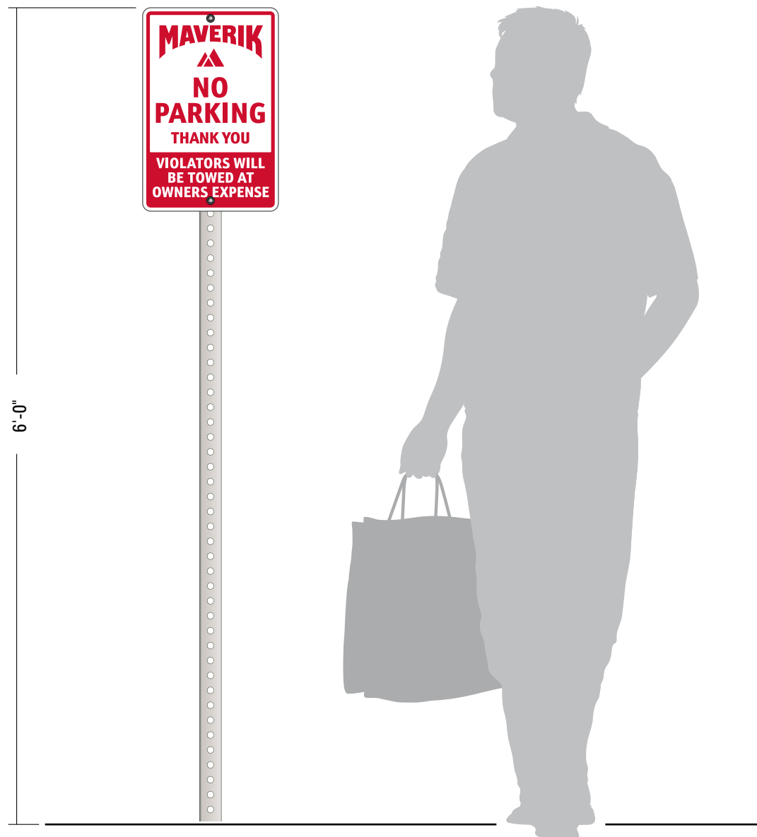
2 SIGN 12 (A-W) - SINGLE FACE SIGN PANEL (TYP.) SCALE: 1" = 1'-0"
