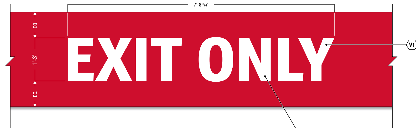
1 SIGN 09 (A-C) FUEL CANOPY VINYL SIGN 3EA. SCALE: 3/4" = 1'-0"
