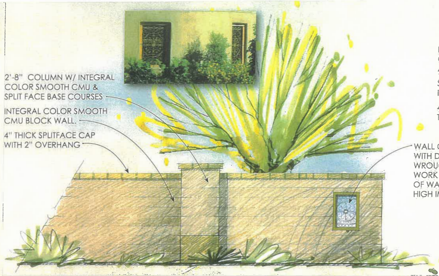
SECONDARY WALL with DECORATIVE ENDWALL DETAIL
